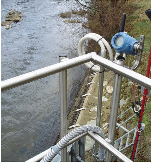
SENSORS MEASURE WATER TEMPERATURE AND TRANSMIT THE DATA WIRELESSLY TO A BASE STATION
